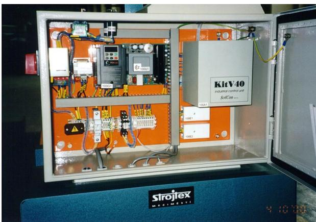
The control system uses information from strain gauge sensors about the fabric tensile stress to control asynchronous driving unit by frequency inverter and it sets required tension of the fabric. The tension of the fabric can be programmed in ten steps, it means a customer can program different fabric stretching force for parts of winding. The control system contains ten programs for different sort of fabric at maximum. The control system can measure the fabric
